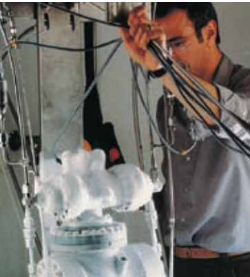
Testing leakage in the Vulcain engine Chamber Valve under cryogenic temperatures.
