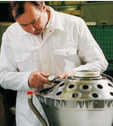
Assembly of the bearing compartment module for the CFM56 engine.
