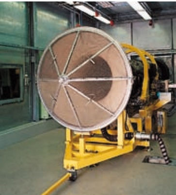
Turn-key test facility designed and installed by Techspace Aero at the Florennes Air Base. The Belgian Air Force operates F16 aircraft powered by F100-PW engines.
